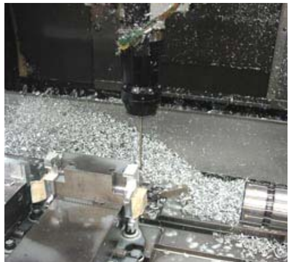
MP10 spindle probe setting the component for further machining operations
