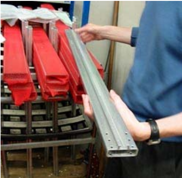
Ejection seat guide rails – wall thickness, gauged with the spindle probe, is critical along the full length
