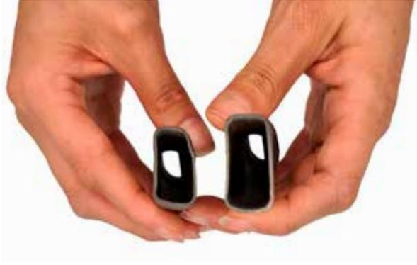
Comparison of a hand-welded and metal 3D printed chainstay bracket
