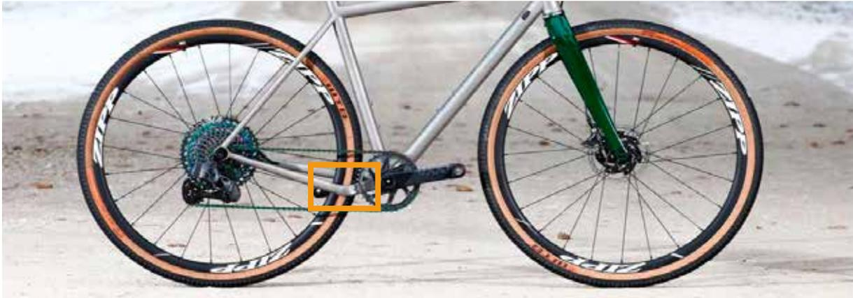
Highlighted inside of the orange rectangle, shows the location of the 3D printed titanium chainstay bracket
