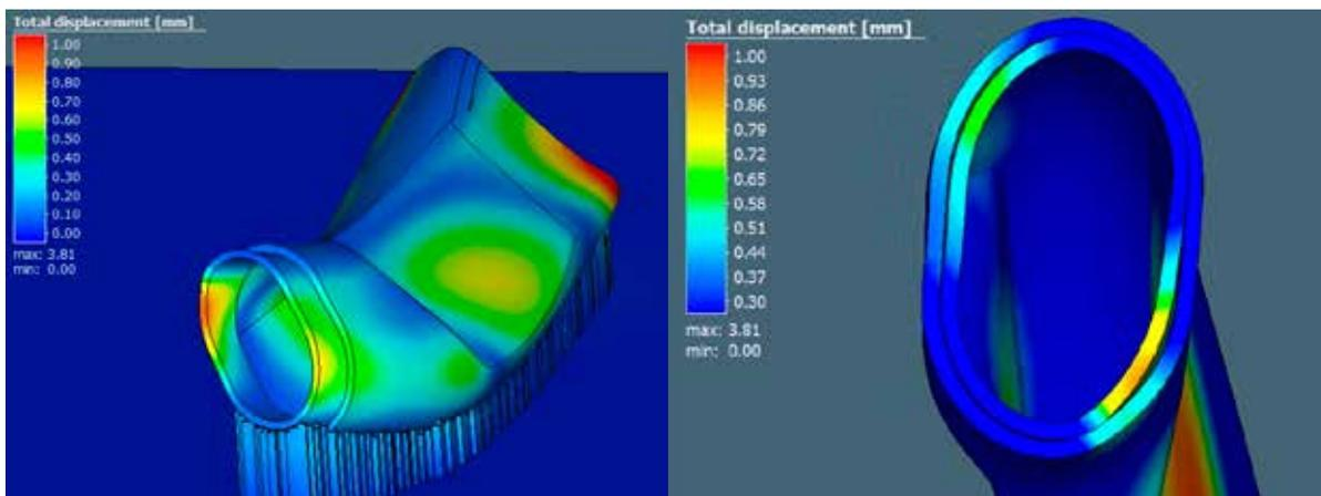
Analysis of the additively manufactured titanium chainstay bracket using Simufact software
