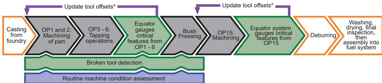
\* Offset updates are automatically applied using IPC (intelligent process control) software which uses dimensional data to feedback offset updates to CNC controllers. Updates could alternatively be applied manually based on the inspection data displayed in Process Monitor.
