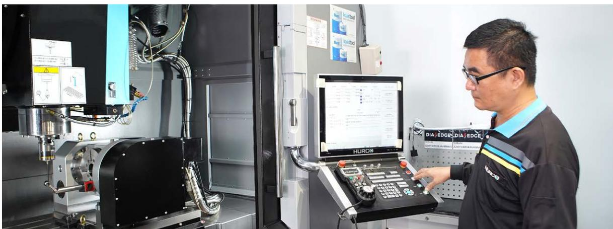
Hurco also uses the Renishaw RMP600 high-accuracy touch probe for workpiece inspection and job set-up
