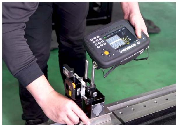
XK10's display unit to collect, analyse and record measurement data
