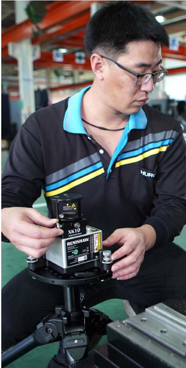
Hurco using XK10 alignment laser system
