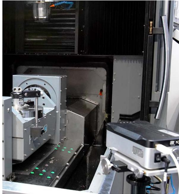
Hurco also use Renishaw’s XL-80 laser interferometer system and XR20-W rotary axis calibrator
