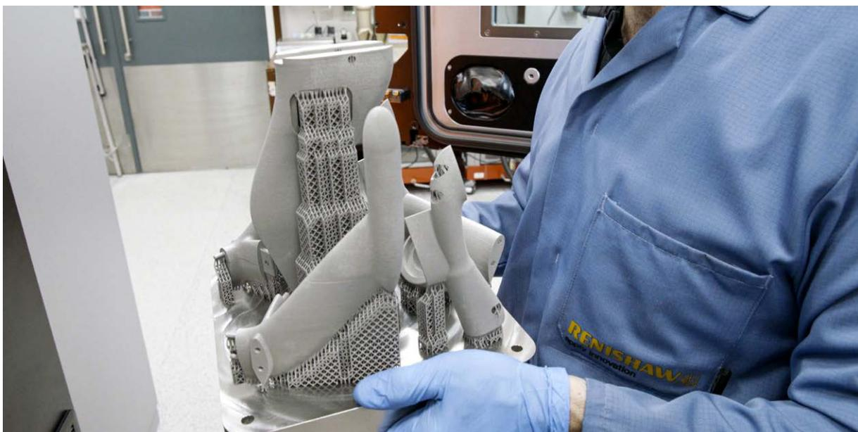
Prototype handlebar components after removal from a Renishaw RenAM 500Q additive manufacturing system
