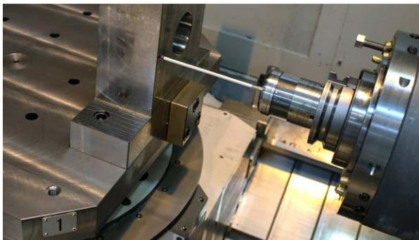
The RMP60 touch probe in use on a machine tool at FMC Technologies
