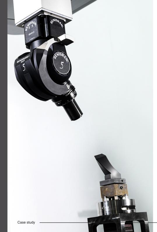
With the multi-sensor capability of its REVO® system, AGILITY® enables DMNC-EDM to conduct a variety of inspections, such as measuring the profile and form of critical parts using contact measurement and then inspect the geometric features of the parts' profiles using vision technology.
