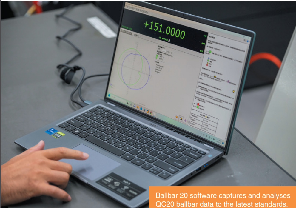
QC20 ballbar inspections proactively assess each machine's condition.
