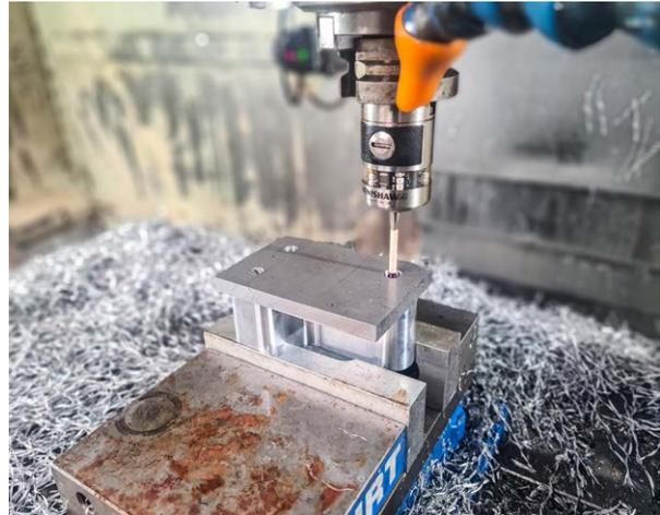
Workpiece set up and inspection using Renishaw's OMP40-2 optical transmission probe
