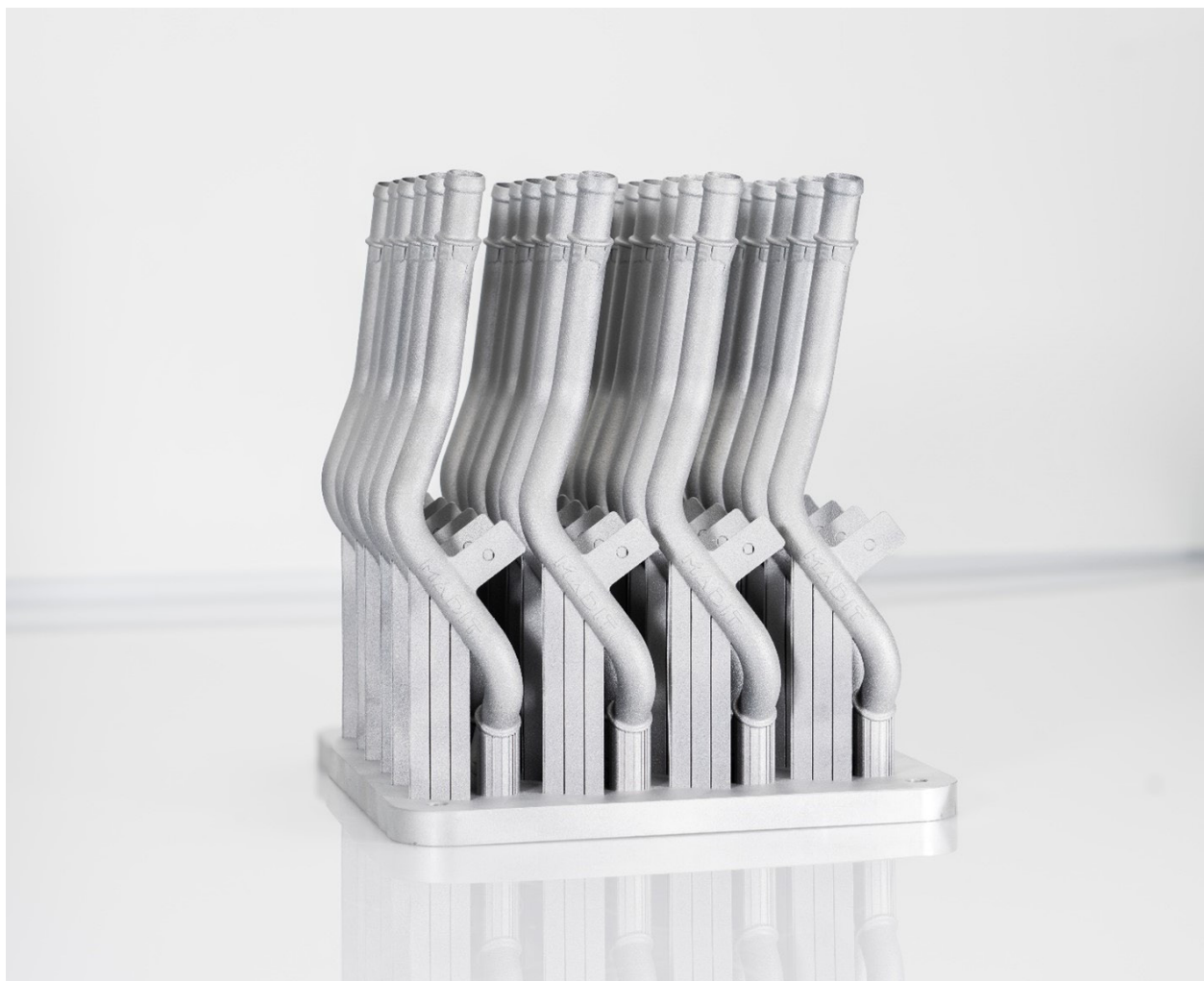
Figure 3 Case study components attached to build plate
