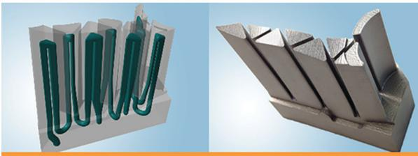
Cooling channels just below mould tool surface reduce press cycle time
