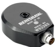
The material temperature sensor is used in applications that require scale, work-piece or machine structure compensation. The sensor contains a calibrated thermistor to monitor material surface temperature in the range of 0°C to 55°C. The temperature reading is converted into a digital signal inside the sensor, which reduces susceptibility to noise when the reading is transmitted to the RCU10.
