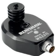
The air sensor is used in applications that require refractive index compensation. The sensor contains a calibrated thermistor to monitor ambient air temperature in the range of 0°C to 40°C. The temperature reading is converted into a digital signal inside the sensor, which reduces susceptibility to noise when the reading is transmitted to the RCU10.
