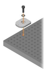
4. Affix the remaining parts of the tool setter to the base plate.
