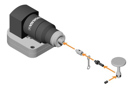
2. Connect the opposite loop of the captive link to the disc stylus.
