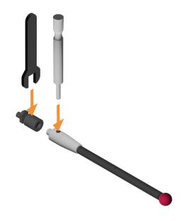
2. Using the C-spanner, attach the break stem and stylus to your tool setter.
