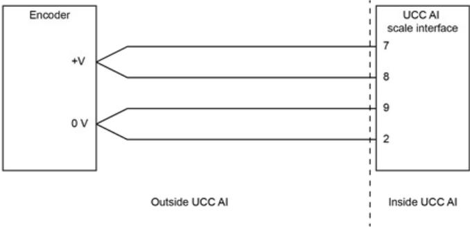
The scale inputs support a quadrature waveform with a minimum edge separation of 50 ns, which equates to 20 million counts per second with an ideal waveform.
