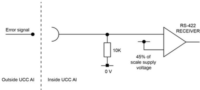
The UCC AI supports the error signal provided by Renishaw's digital incremental encoders. The UCC AI can also detect tri-state conditions on the A and B signals. If the error signal is not integrated into the connected encoder, then the user should connect pin 3 (Error -) to pin 7 (+V scale).
