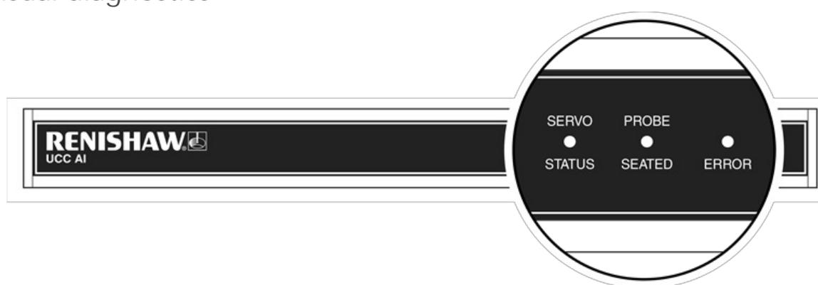
A visual indication of the system status is provided by three LEDs on the front panel, providing assistance in diagnosing and rectifying system faults.
