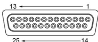
The connection on the UCC AI is a 25W D socket with the following connections:
