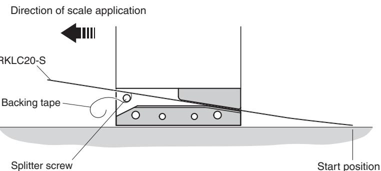
9. During installation make sure the scale adheres to the substrate by pressing lightly.
