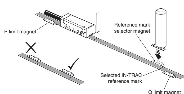
**NOTE:** The reference mark selector and limit actuator locations are correct for the readhead orientation shown.
