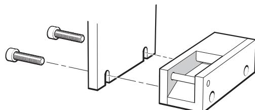
**NOTE:** The scale applicator can be mounted in either direction to install the scale more easily.
