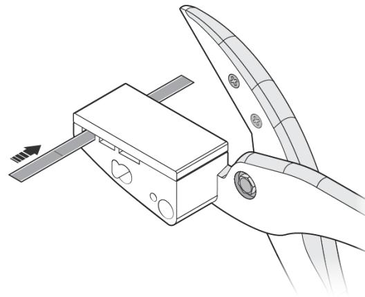
Hold the scale in place and close the shears in a smooth motion to cut through the scale.
