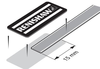
**CAUTION:** Wipe excess epoxy away from the scale as it may affect the readhead signal level.
