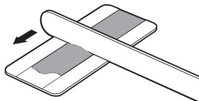
3. The end clamp features two small regions of contact adhesive. These will temporarily hold the end clamp in position while the epoxy cures. Remove the backing tape from either side.
