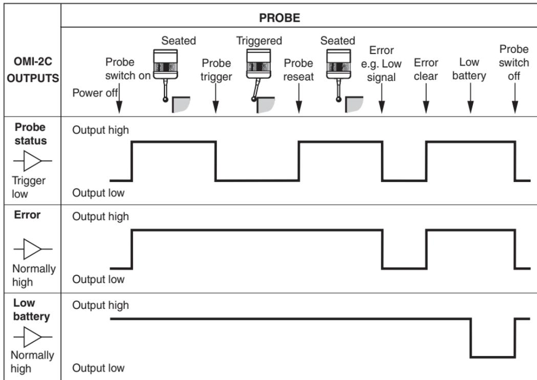
The output signals from the OMI-2C must be compatible with the machine control input.
