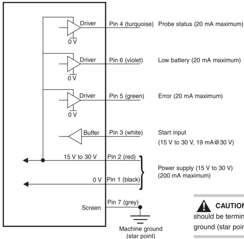
**CAUTION:** The power supply 0 V should be terminated at the machine ground (star point).
