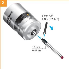
Removing a broken weak link
