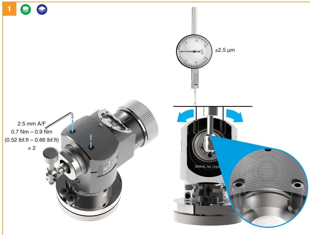
Side-to-side level adjustment is obtained by alternately adjusting grub screws, which causes the probe module to rotate and change the stylus level setting.
