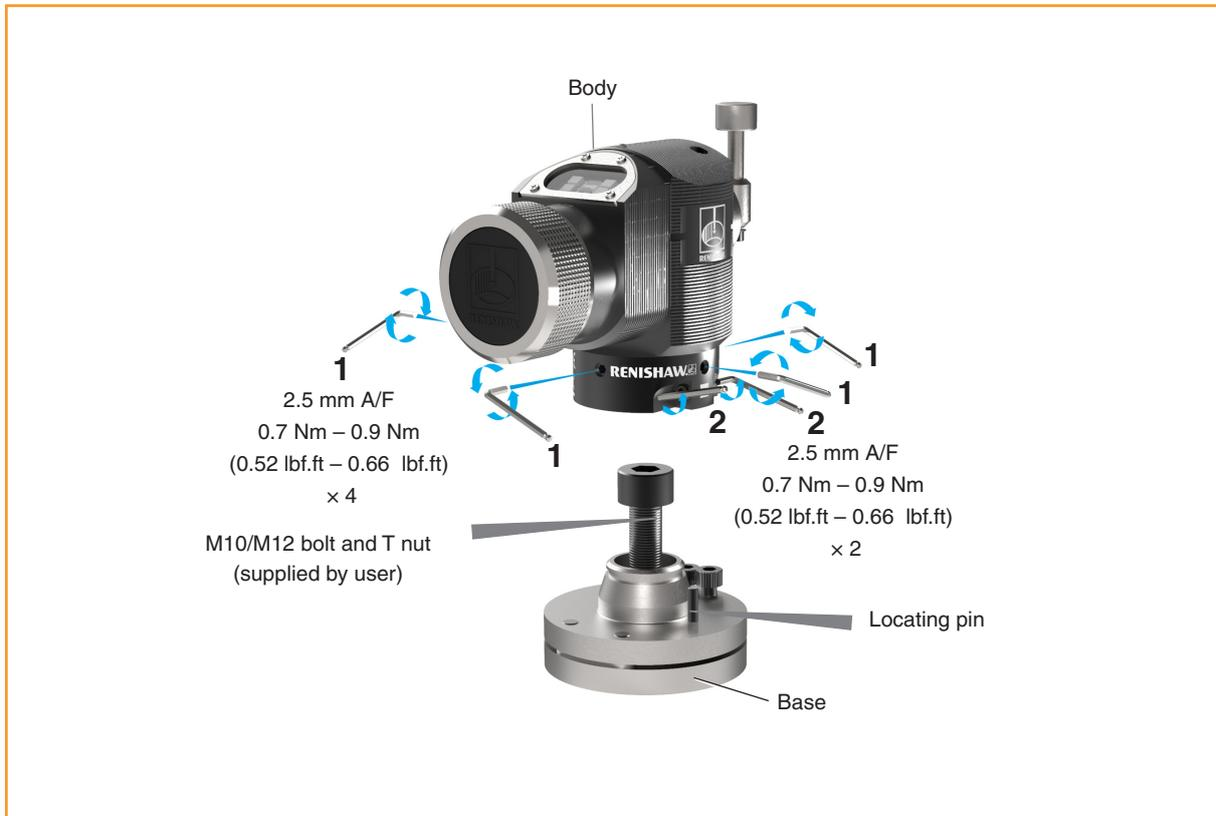
1. Select a position for the OTS on the machine table. Position to minimise the possibility of collision and ensure the optical window faces towards the receiver.
