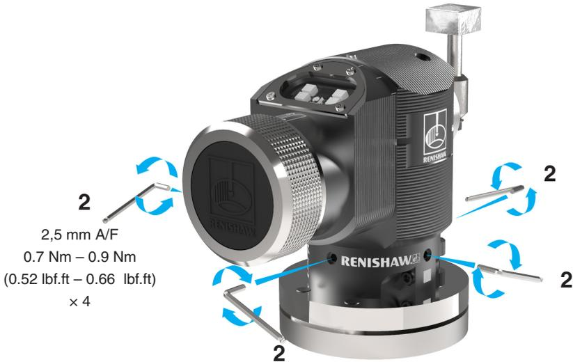
Fully retighten the four body locking screws 2.
