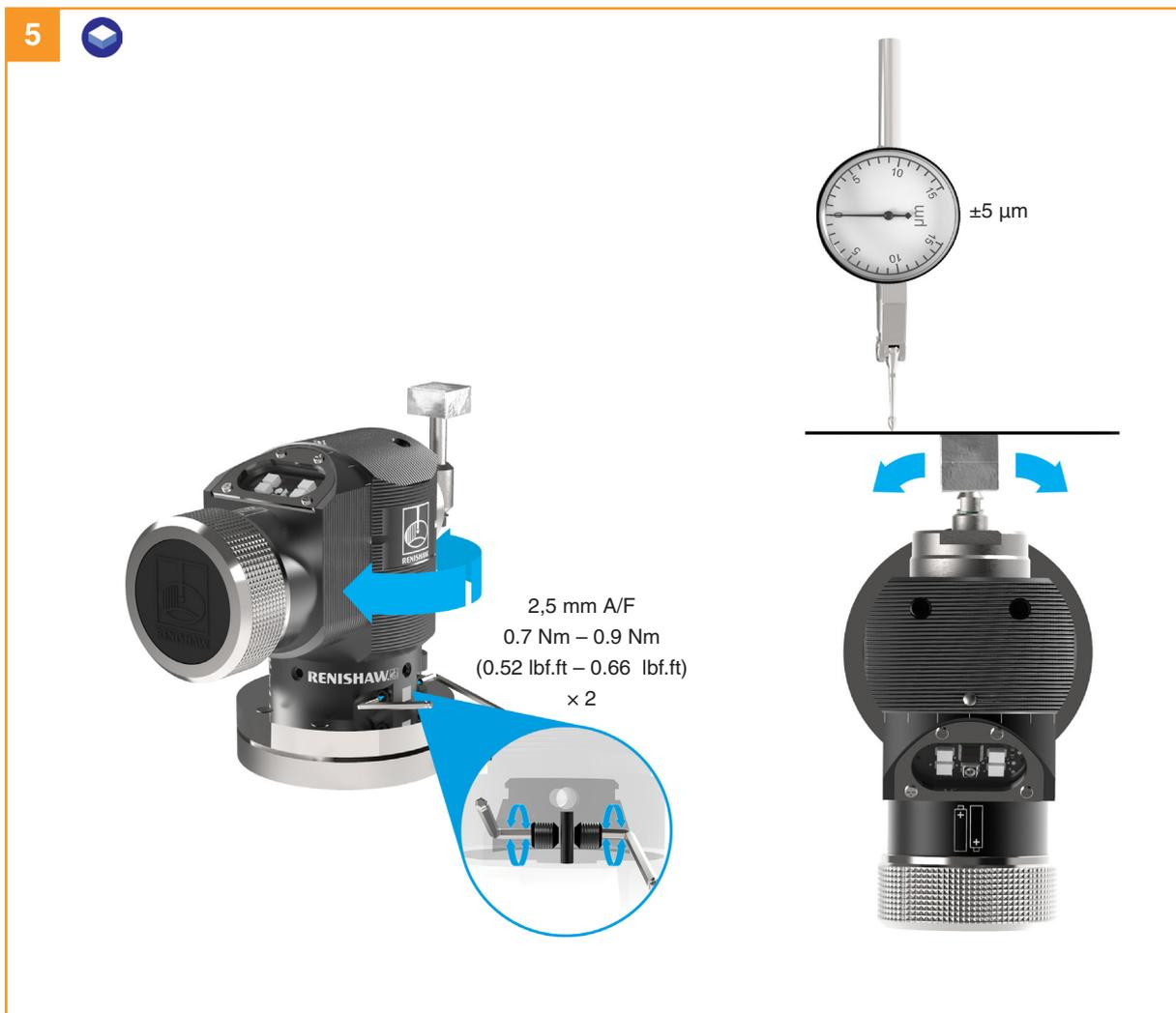
Tighten the opposing grub screws 3 against a locating pin fixed to the base.
