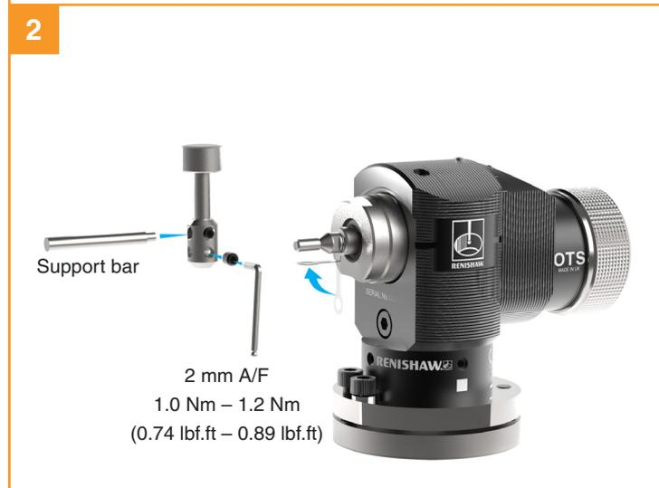
**NOTE:** Always hold the support bar in position to counteract twisting forces and avoid over-stressing the stylus break stem.
