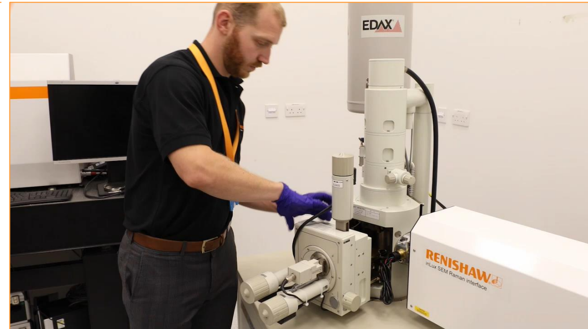
New inLux SEM Raman interface enables simultaneous Raman and SEM analysis
