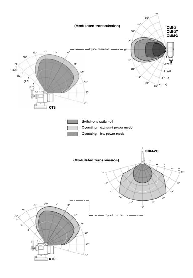
Typical plot at +20 °C (+68 °F) Transmission around probe axis in m (ft)
