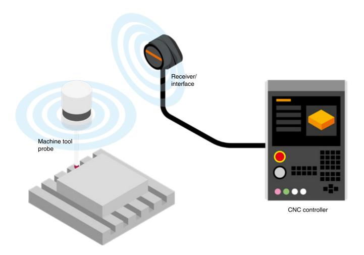
A Renishaw radio transmission system provides communication between the probe and the machine tool controller and comprises the following:
