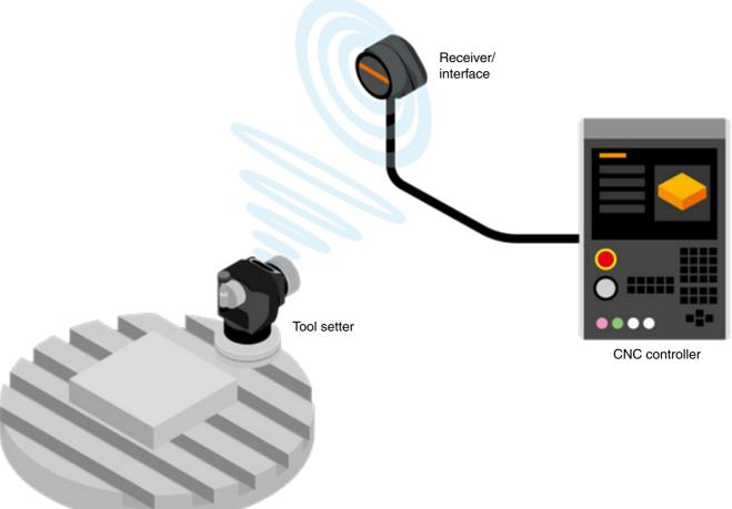
A Renishaw radio transmission system provides communication between the tool setter and the machine controller and comprises the following:
