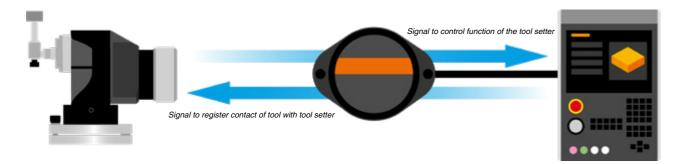
The passage of these signals is handled by a transmission system. The choice of transmission system depends on the type of probe and the type of machine tool to which it is fitted.
