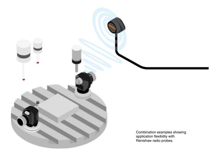
The diversity and capability of Renishaw transmission systems enables innovative multiple probe and tool setter applications and system combinations. The chart below provides some of the typical examples with various transmission types. Further variations of these are possible.
