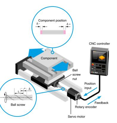
Semi-closed loop system example: a rotary encoder measures rotation of a ball screw and feeds it back to a controller. Linear position along an axis is calculated; 1 revolution = ball screw pitch (L).
