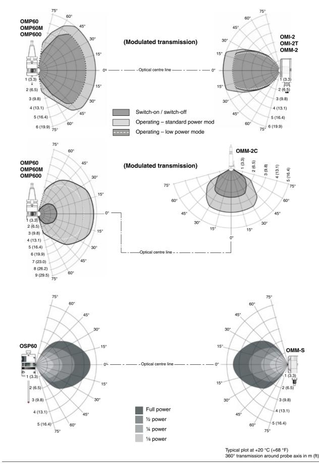
Typical plot at +20 °C (+68 °F) 360° transmission around probe axis in m (ft)
