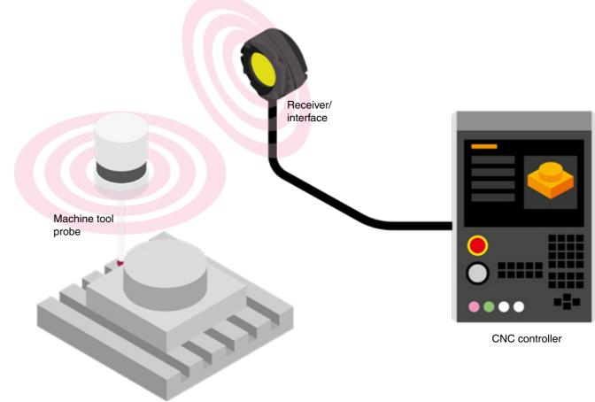
A Renishaw optical transmission system uses infrared technology for communication between the probe and the machine tool controller and comprises the following:
