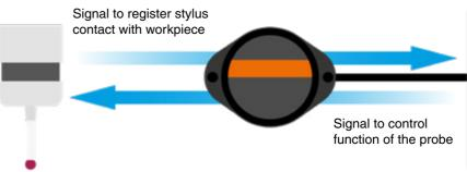
Probes and CNC controllers communicate bidirectionally. The passage of these signals is handled by a transmission system, the choice of which depends on the probe, the machine type and application.
