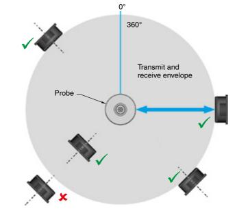
Plan view showing 360° vision envelope and example of positioning options for receivers
