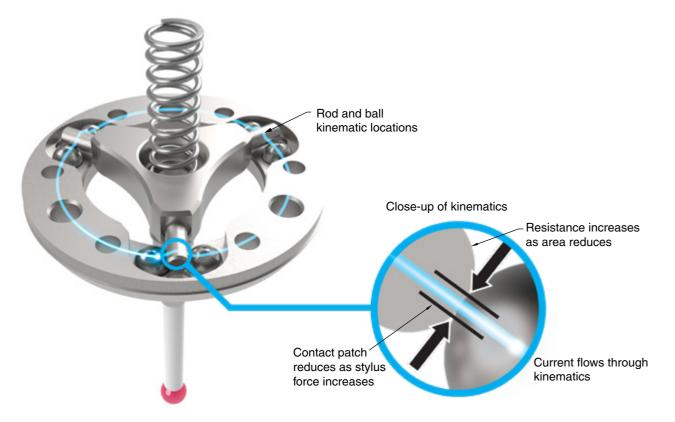
Based on the above kinematic principle, the stages in trigger generation are shown below. Repeatable reseating of the mechanism is critical to this process and fundamental to reliable metrology.
