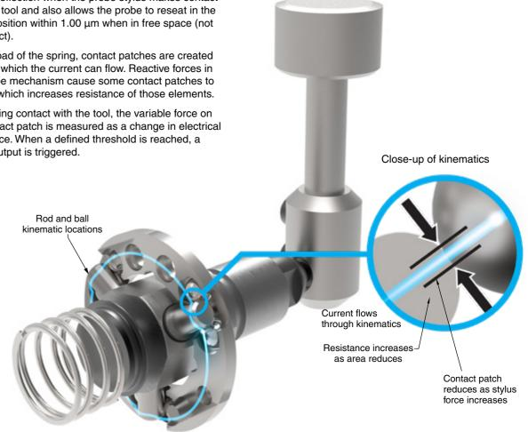
Based on the above kinematic principle, the stages in trigger generation are shown below. Repeatable reseating of the mechanism is critical to this process and fundamental to reliable metrology.
