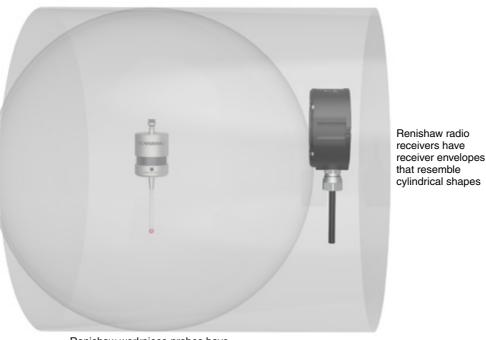
Renishaw workpiece probes have transmission envelopes that resemble spherical shapes
