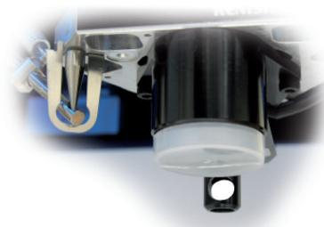
3. There is a magnetic location system that retains the module in position. Align the front of the probe module (indicated by the dot marker above the word 'Renishaw') with the front of the probe body.
