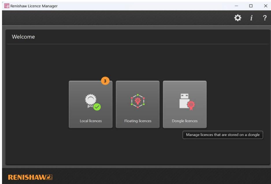
1. Plug the dongle into your computer's USB port. Any licences will appear in the **Manage** tab of the **Dongle licences** screen.
