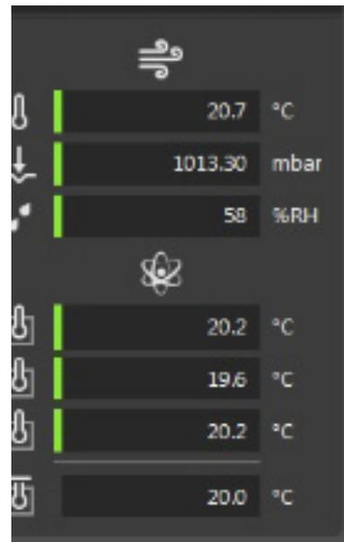
XC compensator readings are taken every 7 seconds, and are used to compensate the laser readings accordingly. Refer to **XC compensator update cycle** for more information.
