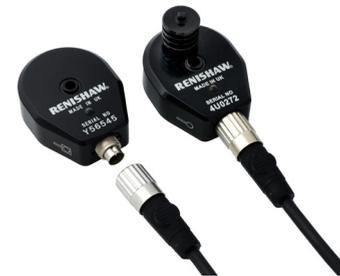
The air temperature and material temperature sensors shown are separate items and are supplied together with communication cables. Each cable has a female threaded connector to join it to the sensor and a male threaded connector to join it to the corresponding socket on the side of the XC compensator.
