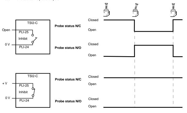
NOTE: Probe status LED will still function when inhibit is active.
